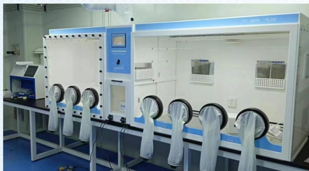
Large Anaerobic Workstation with Integrated Protein Purifier
