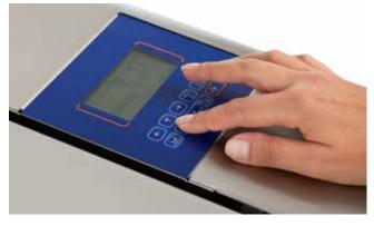
The graphic user interface allows the user to monitor and control the steam sterilizer. It is designed to be user friendly and easy to use. Here is a quick overview of the main sections of this interface.
